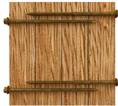
WS6 installed in (4) 1-3/4" Ply
